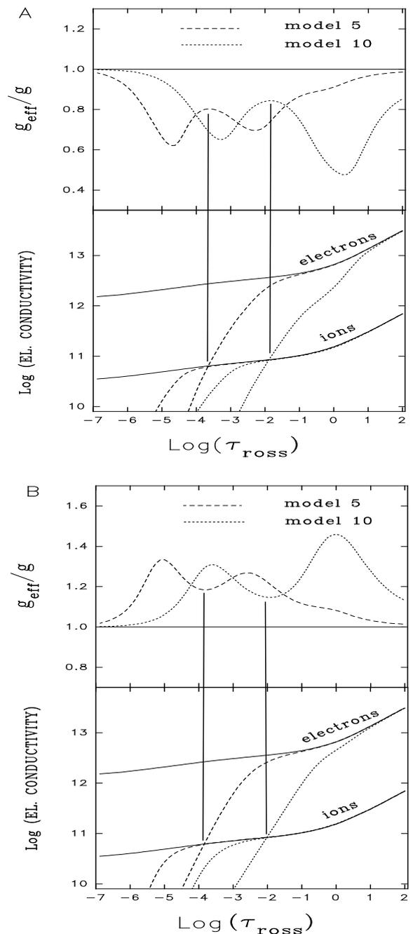
**Fig. 3.** The electron and ion electrical conductivity (logarithmic scale) as a function of the Rosseland optical depth for models No. 5 ( $B_{\text{eq}} = 50$  G) and 10 ( $B_{\text{eq}} = 500$  G) (dashed curves). The electrical conductivity of the electrons and ions in the absence of magnetic field is shown by solid lines. **a)** The outward-directed Lorentz force, **b)** the inward-directed magnetic force.
