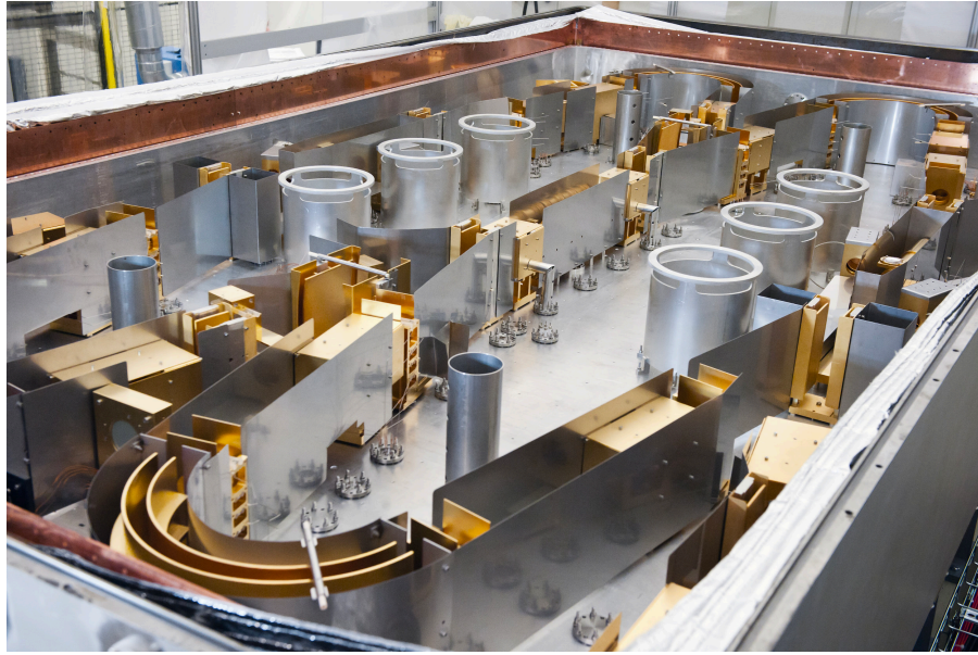
Figure 4: DESIREE (Double ElectroStatic Ion Ring ExpERiment) at Stockholm University. Ions are stored moving in two oblong rings (circumference 8.6 m each), and brought together to collide with each other in the common central section. The particles moving in the same direction to have low relative speeds, typical of stellar atmospheres. The experiment is kept at about 13 degrees Kelvin, or minus 260 degrees Celsius, to reduce background signals. Credit: DESIREE, Stockholm University.
