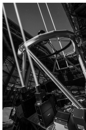
Laser guide stars vid Very Large Telescope i Chile: 4 laserstrålar om 22 Watt vardera
