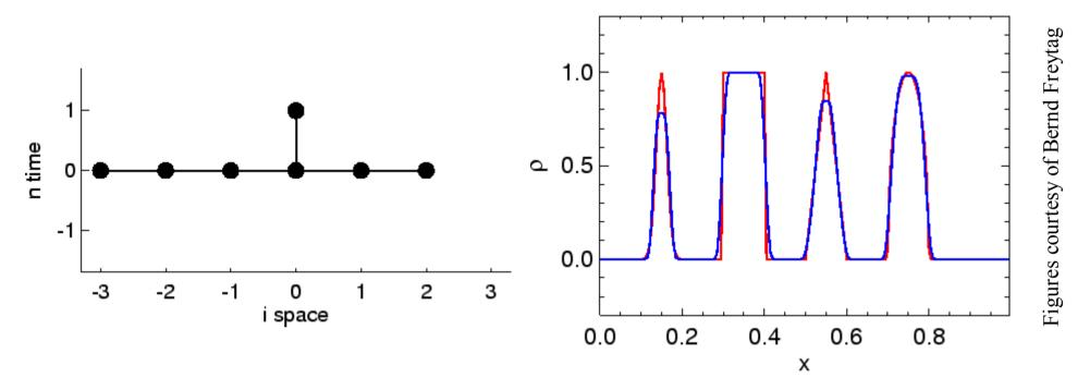
Stencil diagram and test result (initial condition: red, solution: blue) for PPM scheme with piecewise parabolic reconstruction (Colella & Woodward, 1984)
