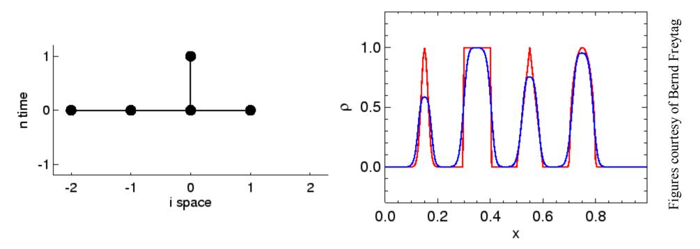
Stencil diagram and test result (initial condition: red, solution: blue) for PLM scheme with van Leer slope-limiter (harmonic mean of slopes)
