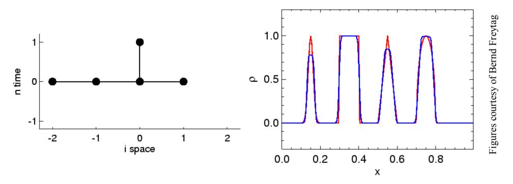
Stencil diagram and test result (initial condition: red, solution: blue) for PLM scheme with Superbee slope-limiter
