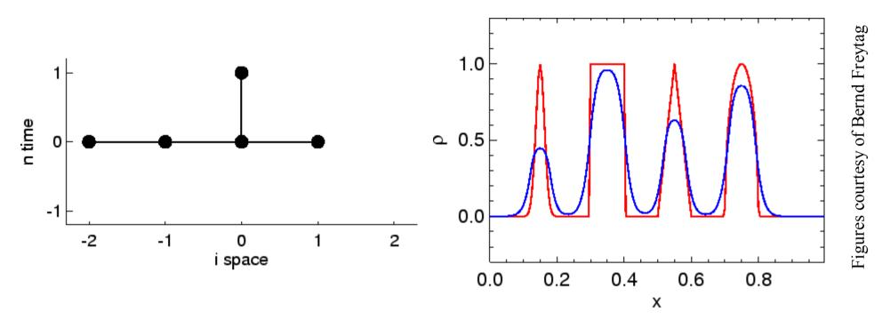
Stencil diagram and test result (initial condition: red, solution: blue) for PLM scheme with minmod slope-limiter
