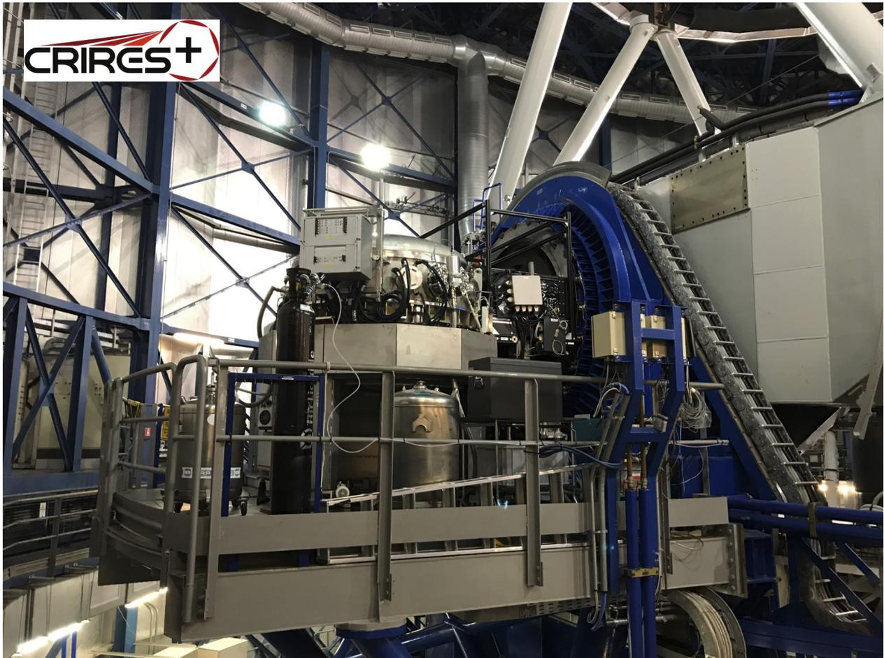
**Fig. 1.** CRIRES<sup>+</sup> instrument in February 2020 installed on Nasmyth focus B of Unit Telescope 3 at the ESO VLT.
