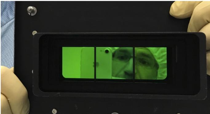
**Fig. 10.** Three CRIRES<sup>+</sup> H2RG detectors arranged as a linear mosaic in the CRIRES<sup>+</sup> specific detector mount including the light baffle.
