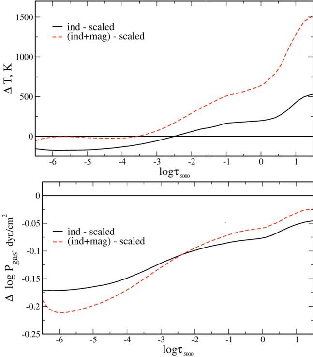
**Fig. 1.** Difference in temperature (*upper panel*) and gas pressure (*bottom panel*) of the models calculated with individual abundances (solid line) and with individual abundances+magnetic field (dashed line) with respect to the reference model atmosphere computed with scaled-solar abundances ( $[M/H] = +1$ ). For all models  $T_{\text{eff}} = 12\,750$  K and  $\log g = 3.8$  are adopted.
