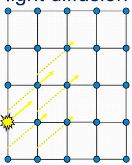
When using short characteristics collimated beams diverge.
