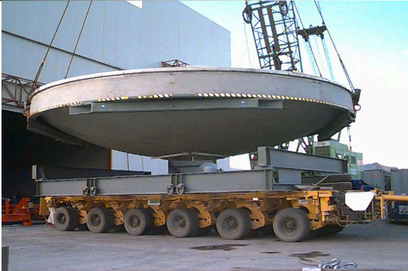
VLT 8.2m mirror coating chamber installed on Paranal
